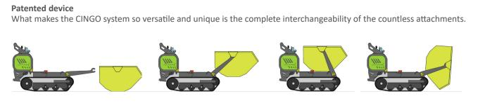
The patented device for rapid attachment connection, which equips the truck with two strong mechanical arms, is the technological base of the CINGO Multifunction. Most of the Multifunction system's attachments are compatible with this device.
